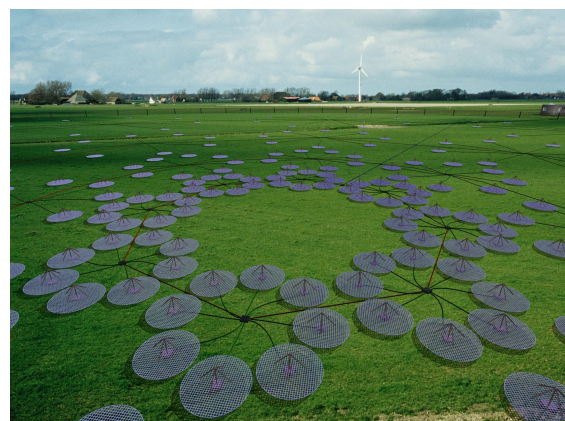
Figure-2: An artist impression of a LOFAR antenna station in the Netherlands (courtesy ASTRON)
